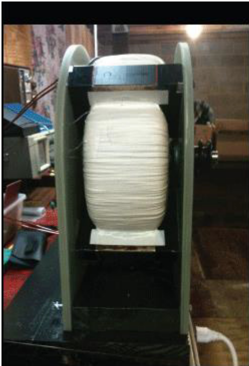
WRAPPED CORE/END PLATES
